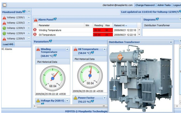
Human Machine Interface displaying transformer parameters
